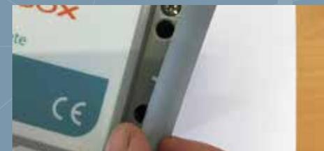
2 Completely loosen the four screws in the cover lid
