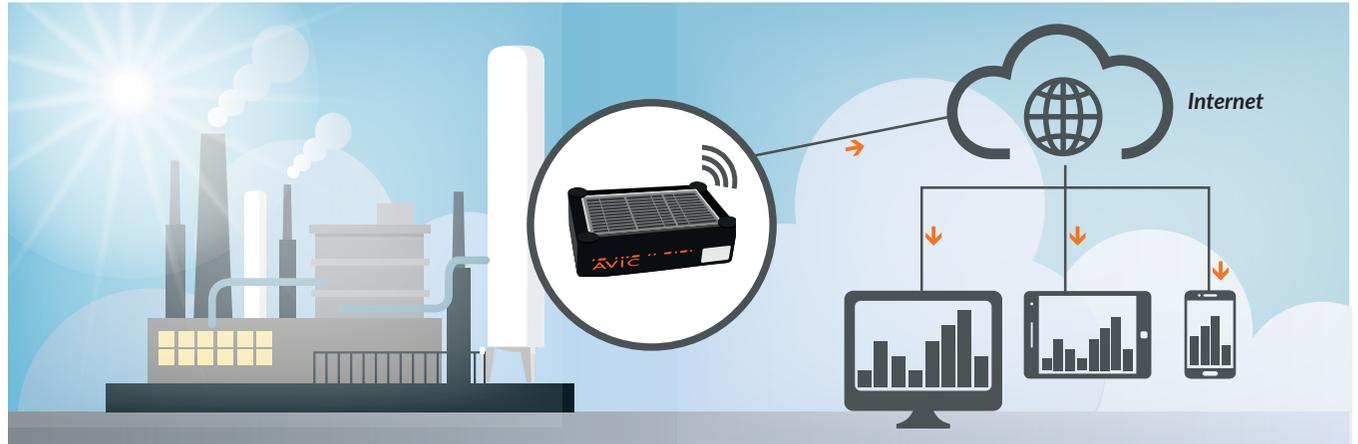
*The information about the level of the tank is sent to the data center using the LegioBox hardware and mobile data communication*
